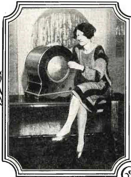
A UNIQUE RADIO RECEIVER. The cone loud speaker in this set acts also as a dial for tuning as well as performing its usual duty. © Fotograms.
