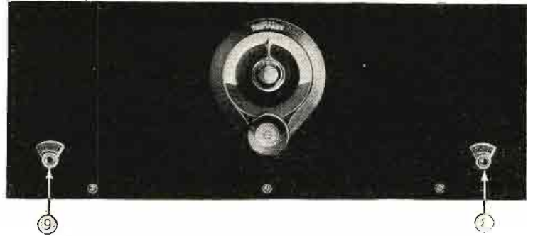
Fig. 5 Note particularly the simplicity of tuning this set. One dial—one control. The locals as well as DX stations snap in and out with great volume and excellent quality, merely by turning the one knob. Jack 9 is for one tube use; jack 8 controls all tubes.
