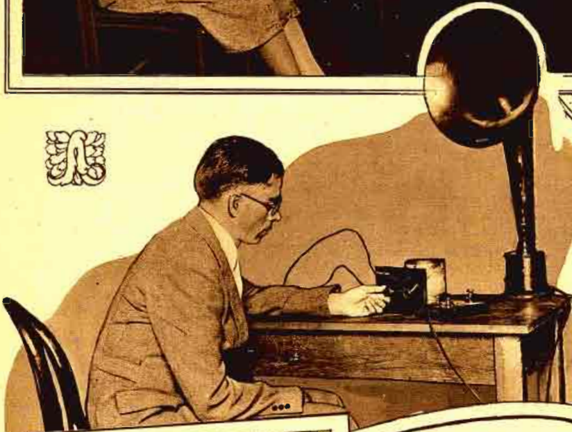
CRYSTAL SET OPERATES LOUD SPEAKER. In the Radio Laboratory of the Bureau of Standards in Washington, Morris S. Strock has succeeded in obtaining signals from a loud speaker using a crystal detector alone. He states that a big antenna and a good crystal are necessary. © Harris & Ewing.
