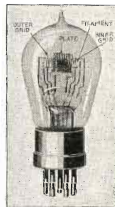
A double-grid vacuum tube that is manufactured in England. It has the same internal construction as that on the opposite page. A special socket is required for these tubes, as they have five connection prongs.
