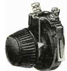
The Perfected C-H Rheostat Designed to radio engineers' specifications. Revolving drum type with one hole mounting. All spring tensions adjusted at factory and undisturbed by mounting. Instrument cannot turn on panel. Very small size—less than 3/4 inch back of panel and narrower than standard socket. Operation smooth and quiet. 6 ohms, 15 ohms, and 30 ohms—perfect control for all tubes and their combinations.
